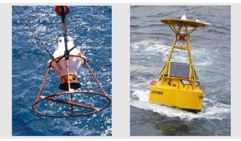
Figure 15: Ocean Bottom Unit (OBU) and buoy
