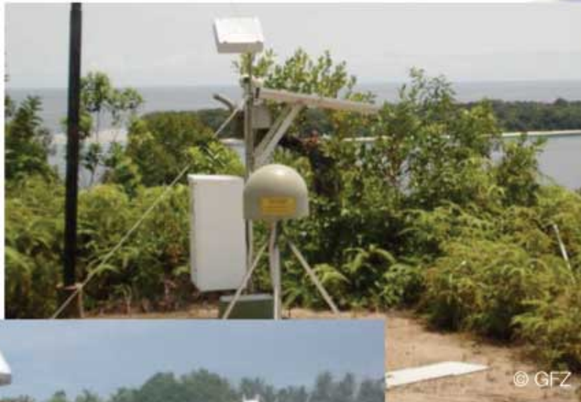
GPS Sensor Station on Land
