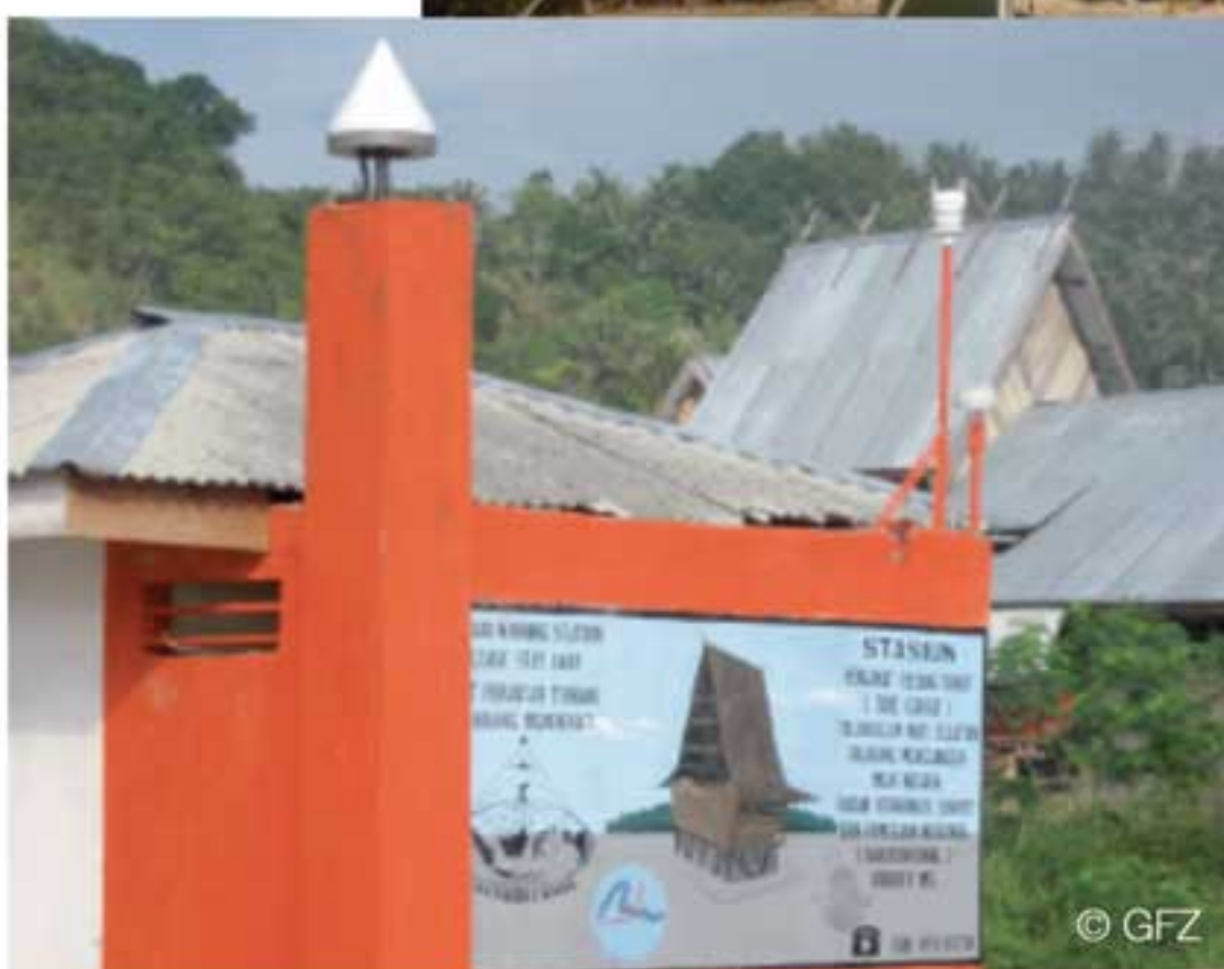
GPS Sensor on Tide Gauge
