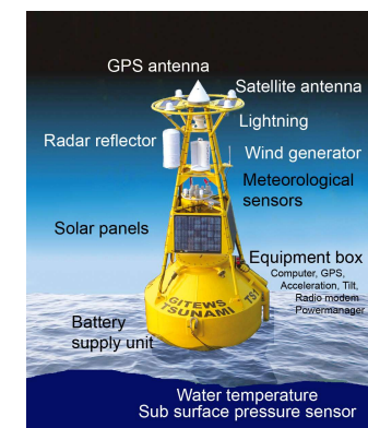
Schematic layout of the GPS buoy
